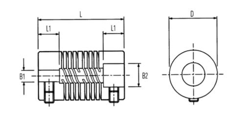
B1: Pre-drilled= 2.0B2: Pre-drilled= 4.00D= 9.5L= 19.6L1= 5.3Max angular displacement = 0.12Max B1 & B2= 4.76Max parallel displacement = 3
